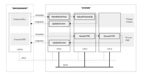
Fig. 1. Overview of the In-car Radio Navigation System
